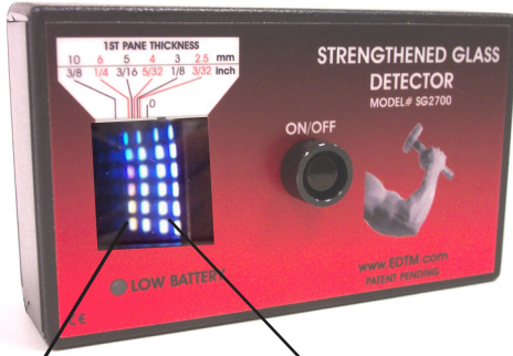
Column 4 on the left: reflection off of bottom surface of 2nd pane
