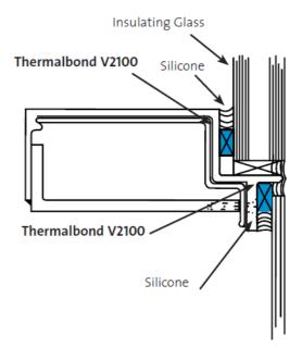
Please NOTE: Thermalbond V2100 is a SPACER material and not intended to be a structural component. **Storage:** Material should be stored at 70°F (21°C), 50% relative humidity.
