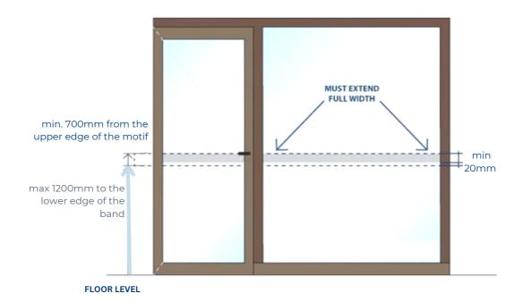
In accordance with the Australian standards AS1288, if the presence of glass in the door or side panel is not made apparent by stiles, rails, transoms, colonial bars, other components of the glazing system, or other decorative treatment, such as being opaque or patterned, the glass shall be marked to make it visible.
