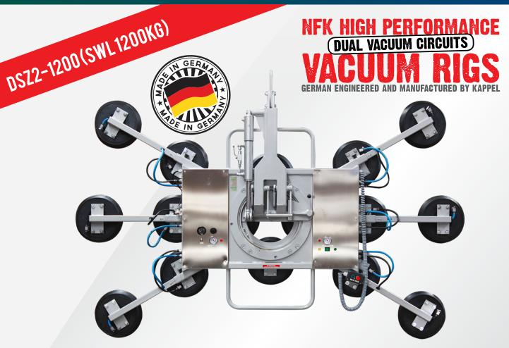
A longer version of the DSZ2-900, this 1200kg SWL rig is packed with features that ensure it will cope with heavy lifting and high repetition workloads. Designed and tested to lift more than twice its rated capacity on only one of the two independent vacuum circuits, the safety margin is theoretically four times the SWL. Six extension arms can be quickly installed and connected to create numerous lifting configurations.
