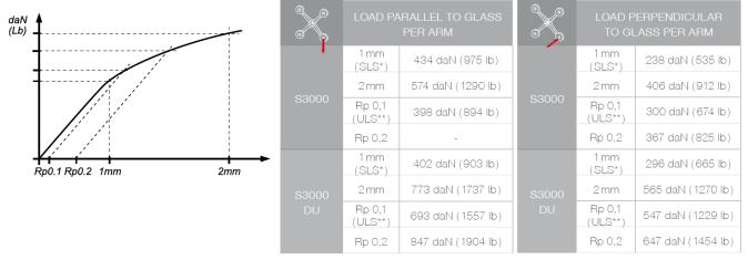
\*SLS: Serviceability Limit State - load at 1 mm deformation \*\*ULS - Ultimate Limit State: load at the elastic limit (Rp0.1) Values are given without factor of safety - Tests available online: www.sadev.com
