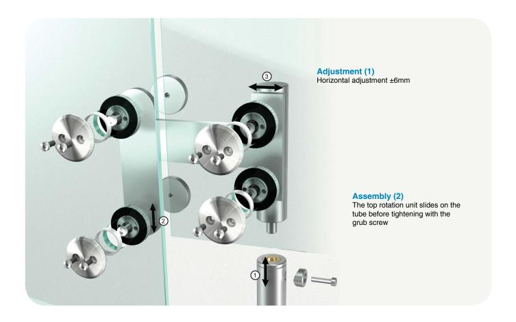
This assembly is used to tie the two fixed glass panels together, in addition to mounting the top pivot above the door. The L plate is fabricated from 10mm thick stainless while the pivot is machined from 40mm solid round bar.
