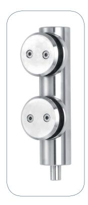
This top pivot is used when a glass high-lite panel is incorporated above the door. Machined from 40mm solid round bar, this pivot appears as an extension of the full length pivot rod.
